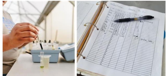
Figure 10. Using a meter to measure pH of the nutrient solution (left), and documenting pH, EC, and other measurements in a binder. (Chris Mullins and Amber Vallotton, Virginia Cooperative Extension)
